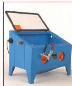
E500 Cyclone Sandblaster Unit Top Opening - 24" x 14" Polythylene Plastic Construction Working Dim: 28" (W) x 18" (D) Trigger Operated: 5 CFM @ 80-100 PSI Dust Collector Not Included
